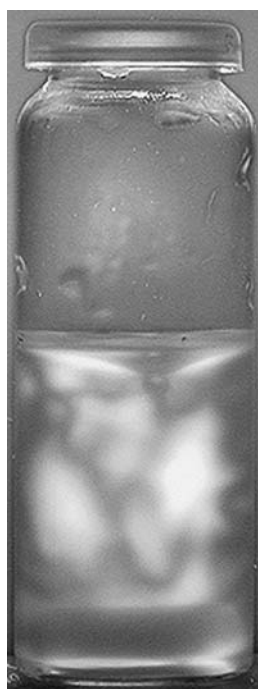
Fig. 4 A suspension of starch, sorbitol and cellulose nano whiskers in water showing flow birefringence when observed through crossed polarizers
